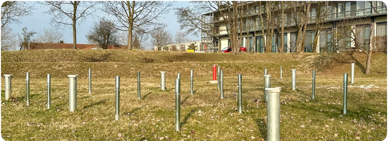
Groundwater monitoring wells at the Teaching & Research Observatory in Pirna-Copitz, with the institute's external campus beyond.
